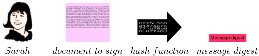
Figure 9: Applying the hash function to the document to generate its message digest.
